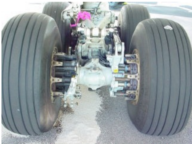
The broken lug (bottom left) of the right MLG
