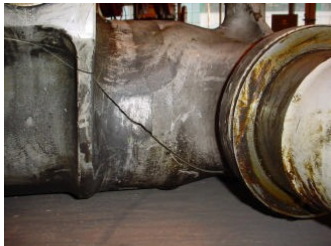
The crack in the right MLG bogie beam
