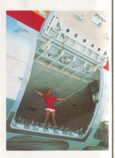
Maximum allowable weight loading of all three cargo compartments is 61,500 lb (27,895 kg) and the maximum space limited volume is 4235 cubic feet (120 cubic meters).
